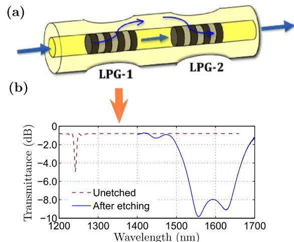
Fig. 1. (a) Schematic diagram of the sensor structure. (b) Transmission spectrum of single LPG.
