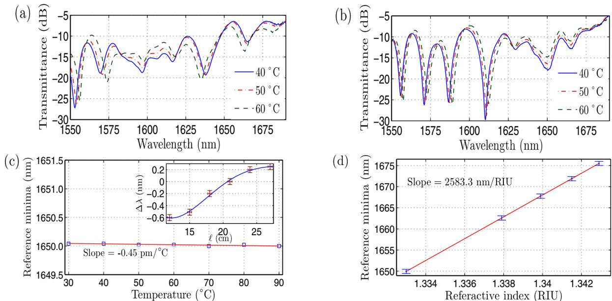
Fig. 2. Experimental transmission spectrum for (a)  $\ell = 18$  cm and (b)  $\ell = 21$  cm. Variation of reference minima near 1650 nm, for  $\ell = 21$  cm, as a function of (c) temperature and (d) ambient RI. The spectral shift, corresponding to maxima/minima near 1650 nm, for different  $\ell$  is shown in the inset of (c) for a temperature increase of 20°C.
