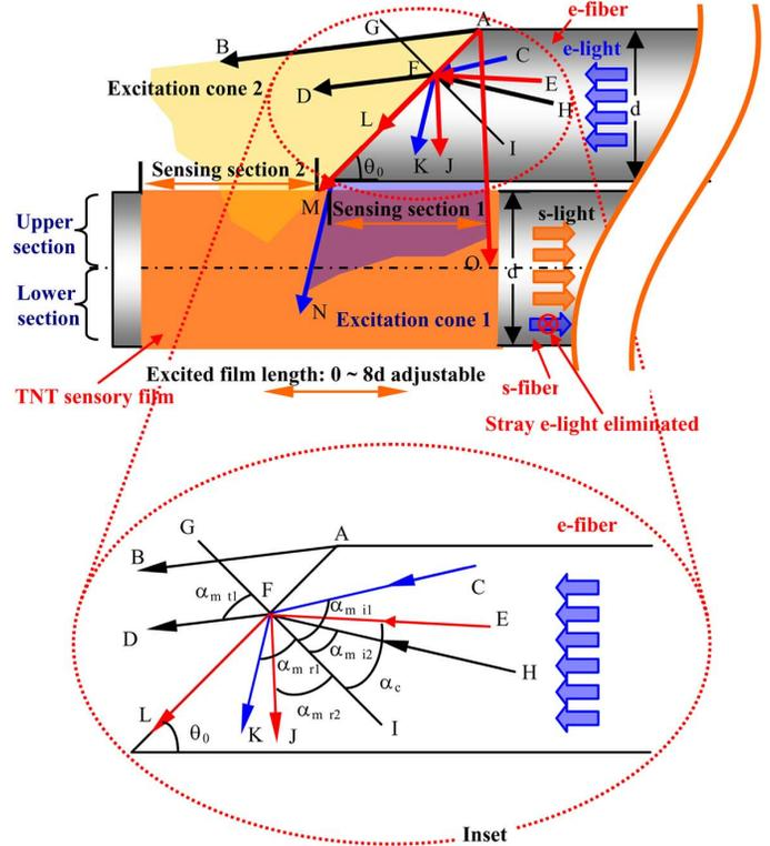
Fig. 2. Theoretical illustration of highly efficient thin-film sample excitation and s-light collection of the proposed LOF device. Adjustable sensing length from 0 to  $8d$  is enabled by sliding either the e- or the s-fiber. Inset: detailed ray tracing to calculate the effective power for sample excitation after departing from the e-fiber core. Note that in principle, the e-fiber delivers the s-light with no stray e-light component.
