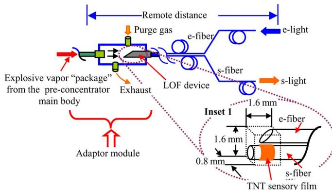
Fig. 1. Example showing an LOF device in the adaptor module. Its tiny internal space ensures high concentration of the sample received from the preconcentrator main body. The received sample “package” is also sent to the LOF sensing area as a “package.” Inset 1 illustrates the architecture and the size of the LOF device. Legend: e-fiber: excitation fiber; s-fiber: signal fiber.
