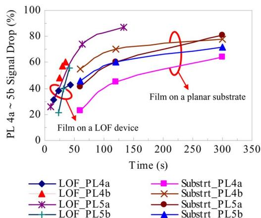
Fig. 4. Experimental results of TNT sensory film fluorescent quenching for devices based on a LOF and a planar substrate. Curves include the results from all four polymers PL 4a, 4b, 5a, and 5b. It is evident that the LOF device has a much faster response than the planar substrate device.
