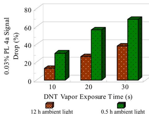
Fig. 6. Ambient light effect on the fluorescent quenching percentage for film formed by 0.03% PL 4a polymer concentration. It is evident that a lengthy exposure to ambient light degrades the polymer film and greatly slows down the quenching response.
