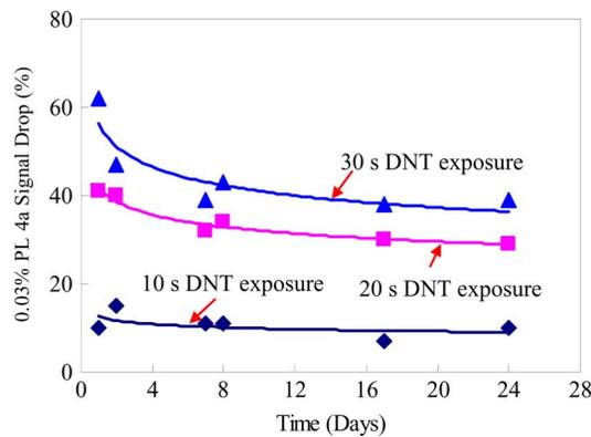
Fig. 7. Evaluation of storage life of PL 4a film over 24 d time following exposure to air containing oxygen but with no ambient light influence. Degradation effect is observable but much less than the ambient light effect in Fig. 6.
