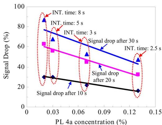
Fig. 5. Fluorescent quenching responses of the LOF to DNT vapor with different thin film thicknesses adjusted by dipping into the polymer solutions with the following concentrations: 0.02%, 0.03%, 0.07% and 0.13% with chloroform as the solvent. INT. time: integration time.
