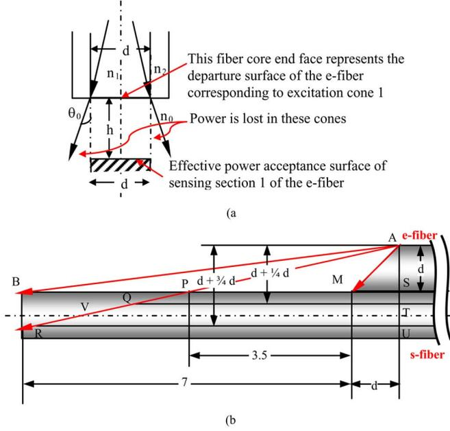
Fig. 3. Theoretical models to calculate the effective excitation power received by sensing sections 1 and 2. (a) Model for both sensing sections for calculating the effective power. (b) Model specifically for sensing section 2. The midpoint P is used to determine the average effective excitation power in this section.
