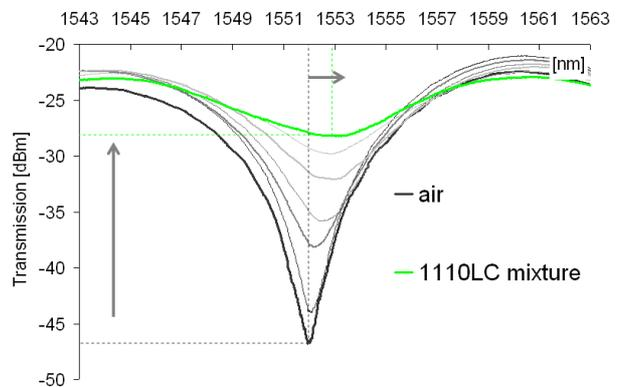
Fig. 2. The transmission spectra of the LPFG when the capillary is being filled by the 1110 LC mixture at room temperature (22.7°C)
