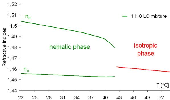
Fig. 1. Refractive indices as a function of temperature for 1110 LC mixture measured at 587 nm (synthesized at the Military University of Technology in Warsaw, Poland.)
