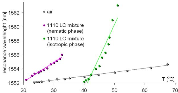
Fig. 4. Comparison of the thermal sensitivity of the resonant wavelength of the LPFG in air and in the 1110 LC mixture.
