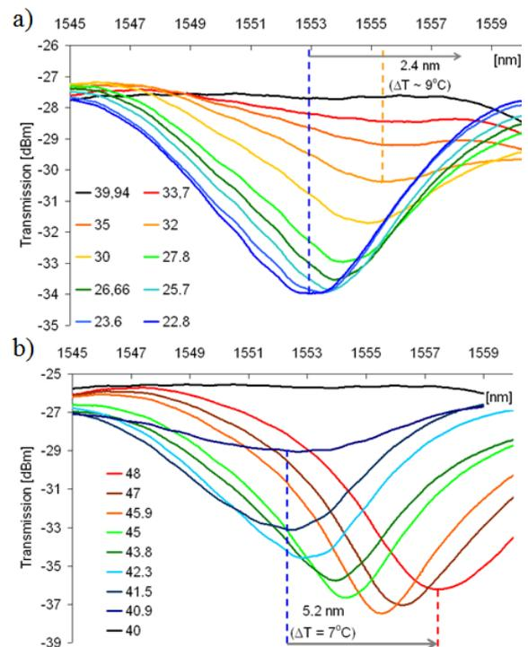
Fig. 3. The transmission spectra of the LPFG with 1110 LC mixture for the temperature range from 22.8°C to 48°C: nematic (a) and isotropic (b) phases of the 1110 LC mixture.
