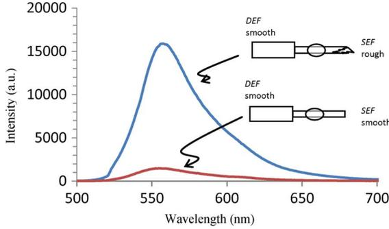
Fig. 6. Output power of fluorescence from  $D$ -end-face (DEF) for two fibers. The higher signal is obtained when the  $S$ -end-face is rough, while the lower signal is obtained when it is smooth.
