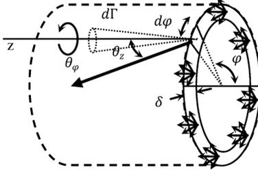
Fig. 5. Random rough surface modeled as a ring-shaped diffuse source near cut-off with a thickness of  $\delta$ .
