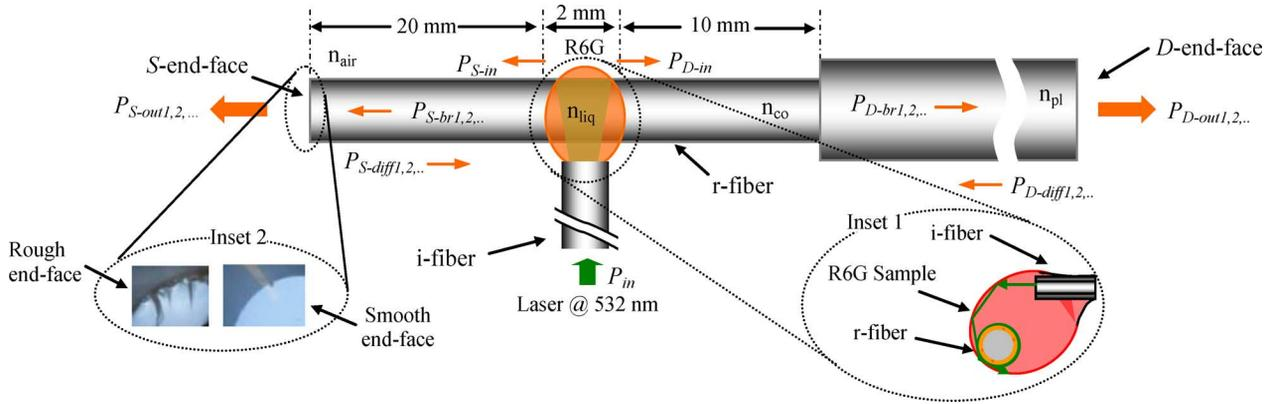
Fig. 1. Powers flow in different segments of a receiving fiber.
