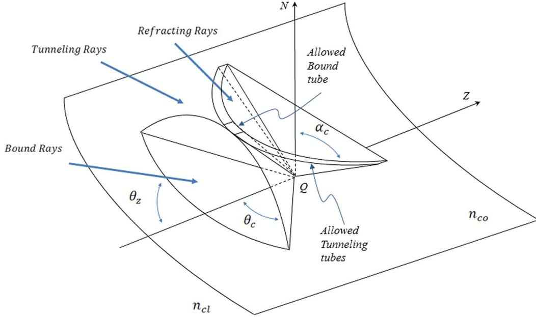
Fig. 4. Tubes which can propagate inside the fiber.
