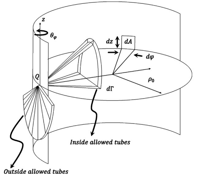
Fig. 3. Fluorescence as a sidewall diffuse source and the tubes which are allowed to penetrate into the fiber from the outside.
