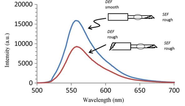
Fig. 7. Output power of fluorescence from the  $D$ -end-face (DEF) for two fibers. In the case of the higher signal, the  $D$ -end-face is smooth while for the lower signal, the  $D$ -end-face is rough. The  $S$ -end-face (SEF) is rough in both cases.
