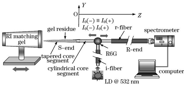
Fig. 1. Optical fiber EW sensing platform for the investigation of the effect of the RI matching gel and the taper on the EW based on fluorescent signal collection.
