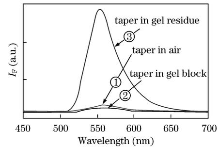
Fig. 2. Experimental results illustrating a significant increase of fluorescent signal collection efficiency when the RI matching gel residue is present on the taper.
